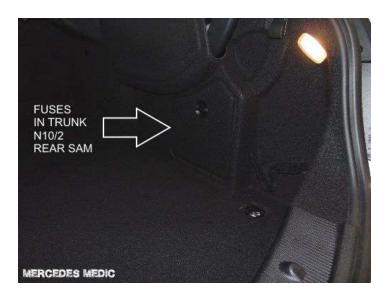
Mercedes-Benz CLS-Class W218, also has a fuse box in the trunk. To access these fuses you will have to remove the cover, usually a carpet cover. This is the rear SAM control module, N10/2.
