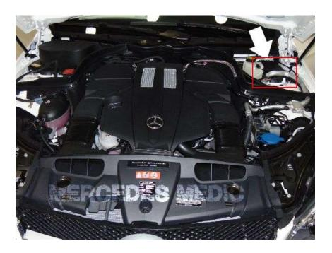
The fuse box in the engine bay contains fuses 1 through 36 and several relays listed below. The fuse box is located on the driver side of the engine compartment. Remove the fuse box panel cover to access these fuses. This is Front SAM control unit, also known as the N10/1 control unit.
